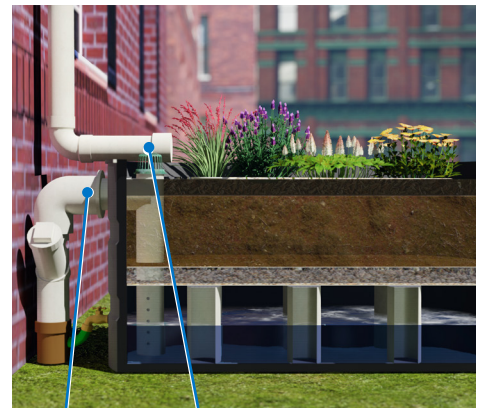
Connected to the roof downspout, these planters slow water down before entering the sewer while irrigating plants and removing pollutants.
