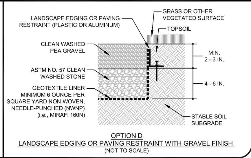
Note: These standard details are not requirements for Rain Check installations. They are meant to provide contractors with different options for permeable paver installations. All installations must meet ICPI requirements for permeable paver installations.
