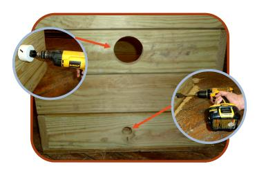
2. Drill hole for underdrain. Using 1-3/8" wood spade drill bit, drill hole with the center point at 3-1/2" from the bottom of the planter, centered horizontally on the short side. (For planters with custom drainage configurations, hole must be drilled at alternate location on planter).
